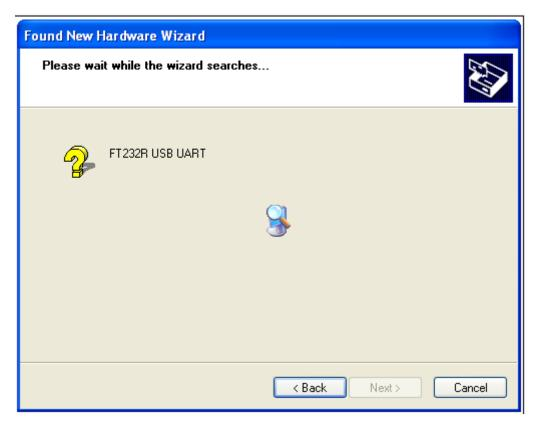
13. When FT232R USB UART is installed, you will be prompted to install USB Serial Port.
